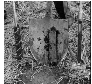
Figure 1. A soil probe, auger, or spade should be used in sampling soils. The spade sample (shown in the center of the picture) should be trimmed as shown with a knife.
