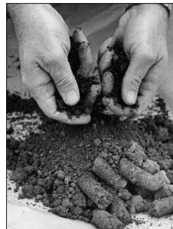
Figure 3. Break up clods while the sample is moist, and spread the sample out to air-dry in a clean area.
