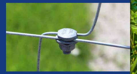
Always connect electrified wires with clamps. Loose connections for result loss of voltage. Connections should NOT be wrapped, but rather clamped together with a high-quality clamp that is designed for high tensile fencing. Never use clamps that constructed of dissimilar metals. Although economy clamps constructed of cast metal are sometimes available, they often fail upon tightening. Saving a few cents on clamps often leads to exponential headaches in the future.
