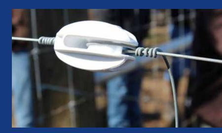
**Terminate hotwires using a bull nose insulator.** At corners, use a bull nose insulator designed for high tensile fencing to terminate hotwires. These can be constructed of either porcelain or fiber reinforced plastics. Avoid using "wrap around" insulators constricted of polyethylene. These types of insulators are convenient, but will eventually will eventually crack and fail, causing shorts at corner posts.
