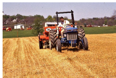
Figure 4. Using a no-till seeder to reestablish forages on a field that has been treated with non-selective herbicide.
