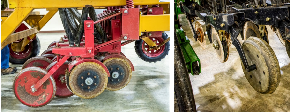
Figure 2. The seeding mechanisms of the Haybuster (lf) and Great Plains (rt) drills. In the Haybuster, the double disks of the row openers are offset so the leading disk can cut through crop residue. The Great Plains uses a separate front coulter to cut through crop residue. The rear press wheels help control depth by limiting the penetration of the row openers where the seed is dispersed.
