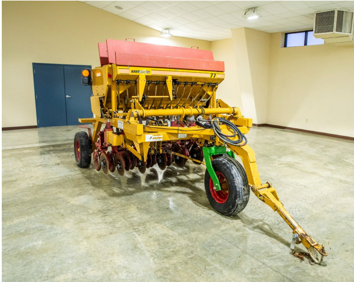
Figure 1. Traditional, furrow-cutting no-till drills are designed to place the desired amount of seed at recommended depths and firm the seed into the furrow with press wheels. When using any equipment, be sure to read and understand the manual and follow its guidelines for maximum success.
