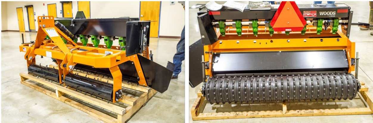
Figure 3. Smaller three-point hitch seeders like this Woods use spiked cylinders or disks (model not shown) to disturb soil ahead of the seeding mechanism. Corrugated rollers in the rear firm the seedbed and help ensure good seed soil contact.
