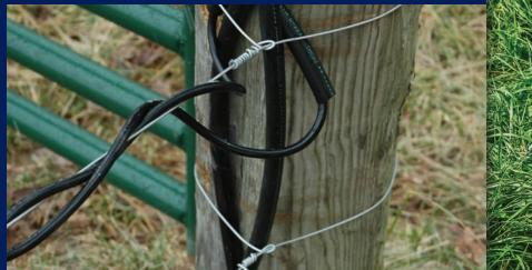
Always use underground cable designed for electric fencing and place it in protective tubing. It is very important to only use underground cable that is designed for electric fence. Never use any product that is intended for residential use. Whenever a cable carrying current is run under the ground, always place it in some type of pipe or conduit that will protect it from future damage. Wires going under gates should be buried to a depth of approximately 1 foot.
