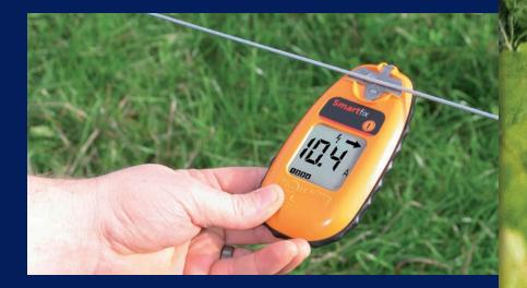
**Use fault finder to monitor voltage and find shorts.** For electric fencing to work properly, a voltage of approximately 5000 volts should be maintained at all times. Shorts in electric fences can cause reduced voltage and can often be difficult to find. A fault finder shows the direction and severity of the of the short. Purchasing a high-quality fault finder is money well spent!
