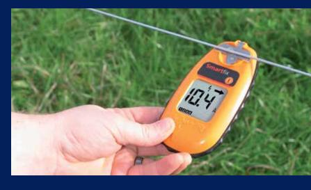
**Use fault finder to monitor voltage and find shorts.** For electric fencing to work properly, a voltage of approximately 5000 volts should be maintained at all times. Shorts in electric fences can cause reduced voltage and can often be difficult to find. A fault finder shows the direction and severity of the of the short. Purchasing a high-quality fault finder is money well spent!
