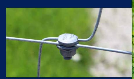
Always connect electrified wires with clamps. Loose connections for result loss of voltage. Connections should NOT be wrapped, but rather clamped together with a high-quality clamp that is designed for high tensile fencing. Never use clamps that constructed of dissimilar metals. Although economy clamps constructed of cast metal are sometimes available, they often fail upon tightening. Saving a few cents on clamps often leads to exponential headaches in the future.
